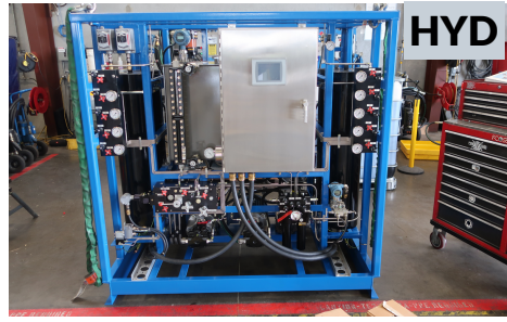
HPU to Drive Fluid Catalytic Cracking Valve Actuators
